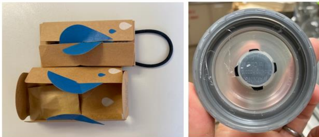
Figure 5.2 Image of cardboard inserts that were inside the bottles Metal A (left) and a cursory visual inspection of a lid from the Plastic C bottle group. Light ribbons of plastic can be seen left over from the manufacturing process.
