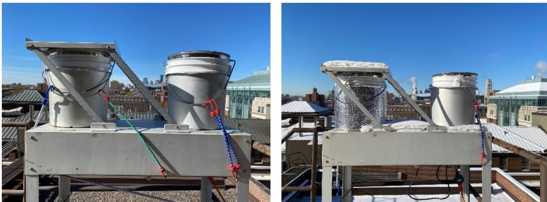
Figure 4.3 Close up of wet and dry deposition sampler collecting during winter (right) and summer (left).
