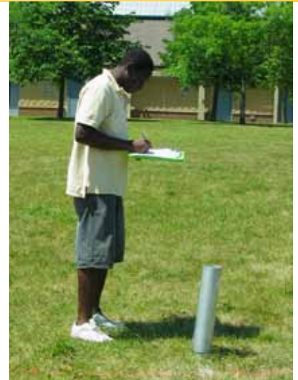
FIGURE 3: High school research assistant Lanre Adekola takes measurements with a Modified Philip-Dunne Permeameter. (Courtesy N. Olson)
