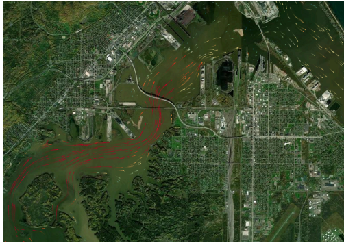
Computer model shows water flow currents in the St. Louis River Estuary.
