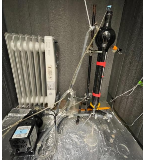
Figure 2-17 Up flow anaerobic sludge blanket reactor setup
