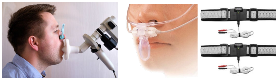
Figure 1. Images of conventional respiration sensing devices including a stationary spirometer (left), a nasal capnography monitor (center), and RIP sensor belts. Source: Images adapted from [14], [15], and [16].
