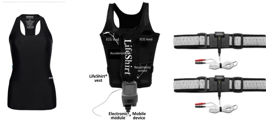
Figure 6. Commercial products using Respiratory inductance plethysmography (RIP) sensors for respiration monitoring. Hexoskin Smart Shirt (left), LifeShirt® (center), Natus® XactTrace® RIP respiratory effort belts (right) Source: Images adapted from [47], [48], and [46]
