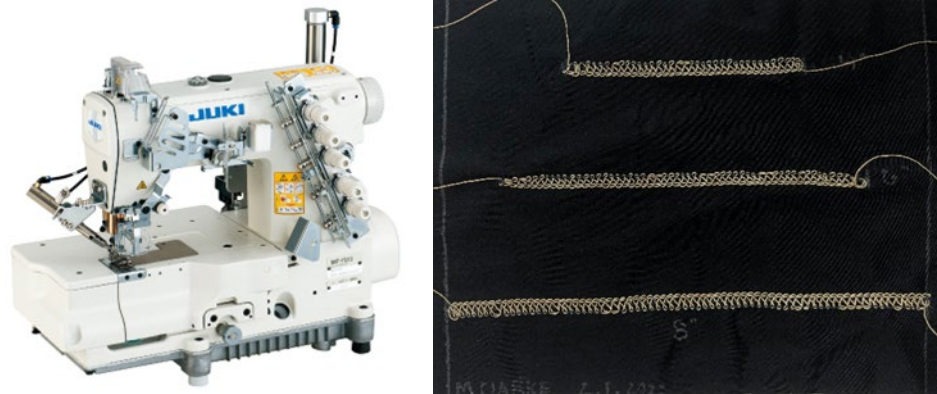
Figure 3. Image of an industrial coverstitch machine used to fabricate the stitched sensor (left) and image of the underside of stitched sensor samples showing the conductive thread (right). Source: Images adapted from [33] and stitched sample provided by author.
