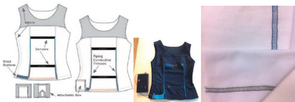
Figure 11. Examples of textile-based piezoresistive sensors include a conductive elastomer sensor (left) and a conductive thread stitched piezoresistive sensor (right). Source: Adapted from [20]-[73].
