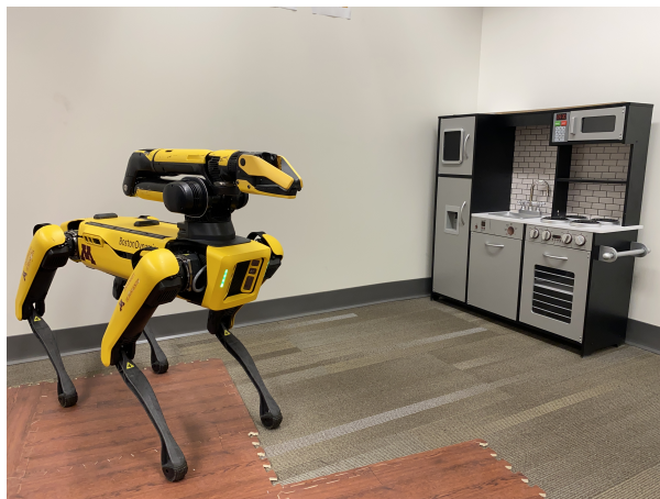
(a) Navigation Success: Robot positioned within 1 meter threshold but inadequate for manipulation
