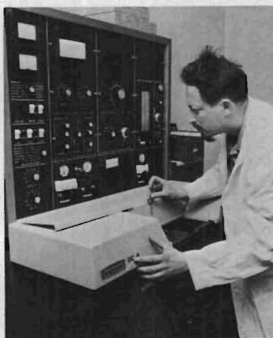
Gas chromatograph unit reduces time needed for performing toxicologic tests from two hours to 20 minutes.
