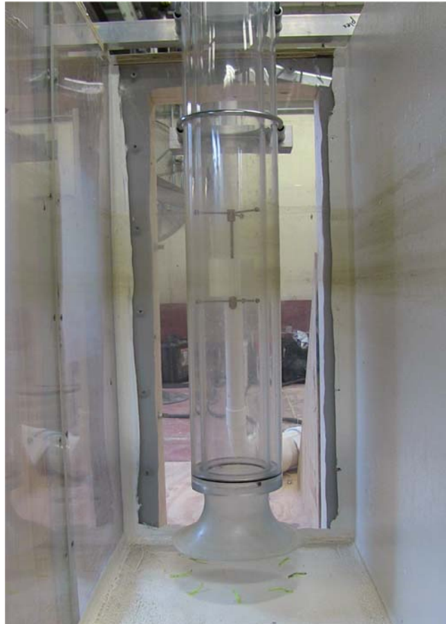
Figure 3: Modeled Vertical Turbine Pump
