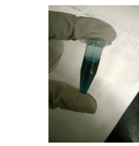
Fig 4. Methylene blue method used for sulfide measurement
