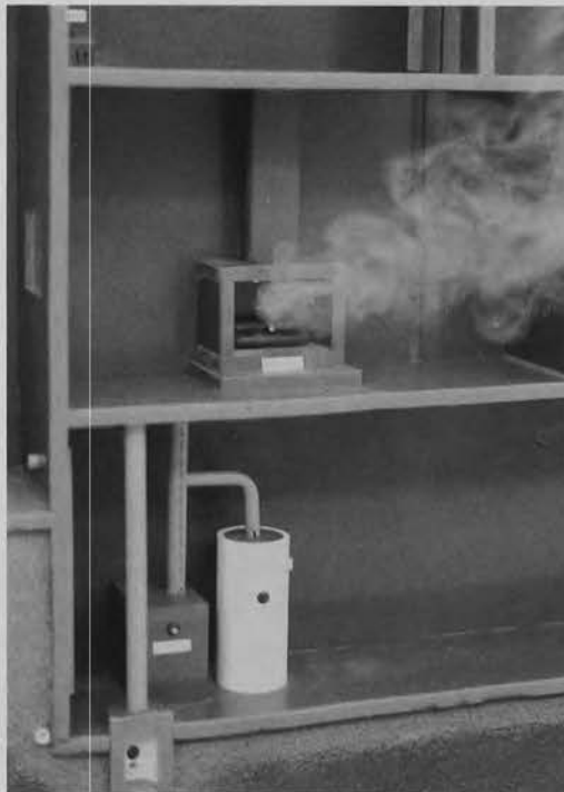
Joe Zulovich (above) and John Fick designed the airflow demonstration model, shown here without the plexiglass face. The model stands approximately 34" wide, 36" tall, and 6" deep, and weighs approximately 90 pounds.
