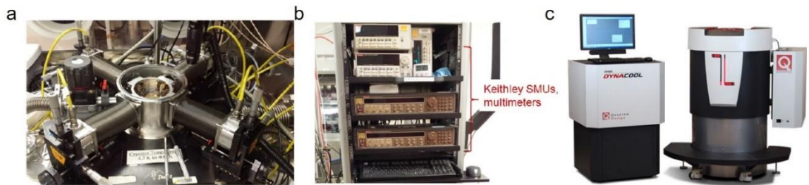
Figure 4.5 Photograph of equipment used in this study. (a) Cryogenic probe station. (b) Keithley SMUs and multimeters. (c) Quantum Design PPMS.
