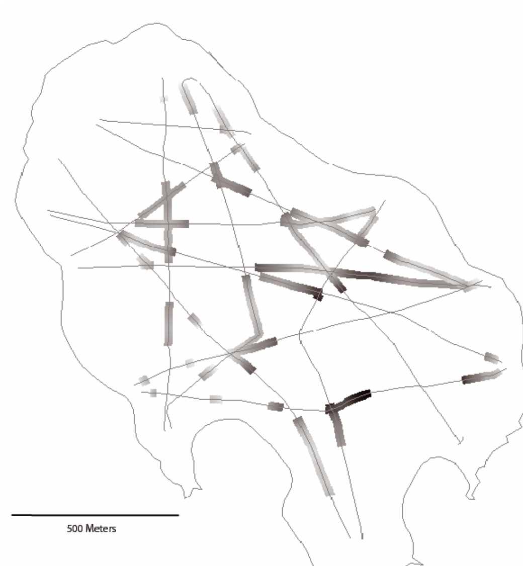
Figure 37a Depth to the unconformity. Map of Elk Lake showing the geophysical lines and depicted with grey scale is the depth to the unconformity as seen in each line. Darker colors represent deeper areas while lighter grey represents shallower depths to the unconformity.
