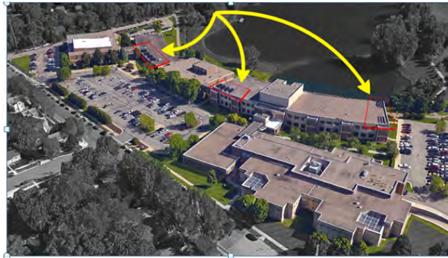
PV panels placement on the selected roofs of City of Chaska government center
