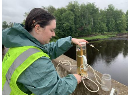
NRRI Field Tech Becca Marston uses a Van Dorn sampler to collect water from the St. Louis River in August.
