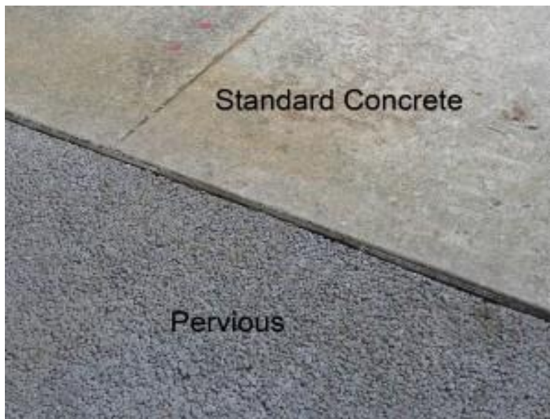
Figure 7 illustrates the aesthetic differences between pervious concrete and standard concrete as a building material option for sidewalks. Figure adapted from source 44 .
