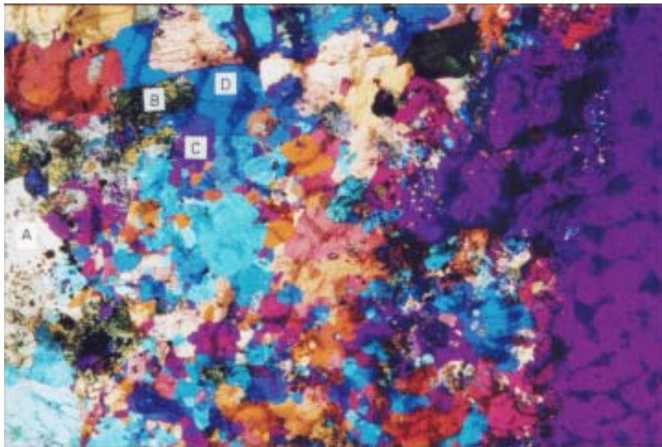
Figure 5. Recrystallization of matrix grains and growth of strain-free rims containing orthopyroxene and biotite on strained porphyroclast cores (A). Some orthopyroxene (O) and plagioclase crystals (C) have straight crystal faces against quartz (D). The quartz shape indicates that it was a late crystallizing phase, hence orthopyroxene and plagioclase developed crystal faces because they grew into a melt pocket. Sample W990763; one wave plate.
