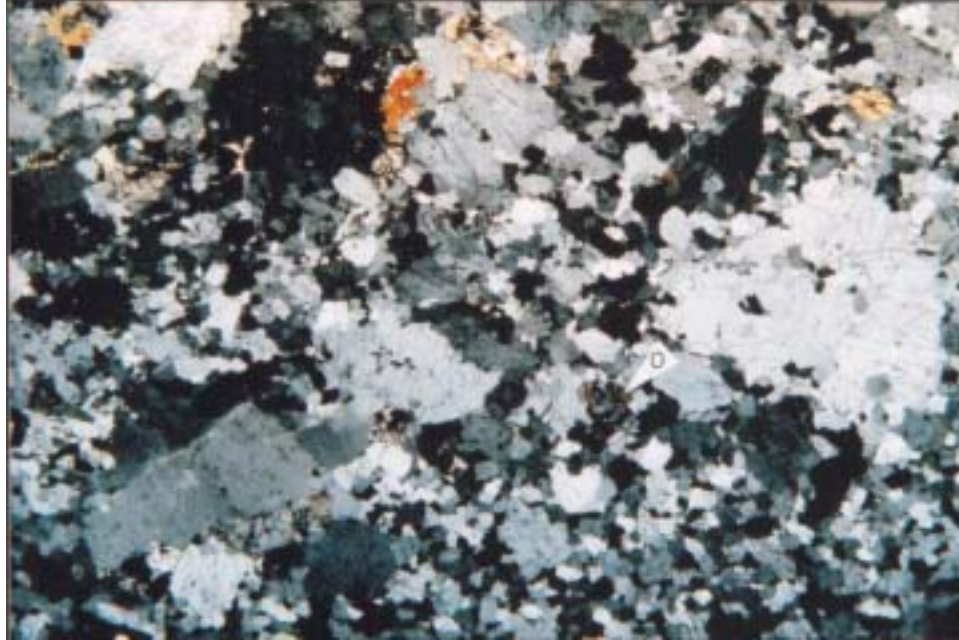
Figure 4. Well developed polygonal texture in the quartz-plagioclase matrix. Orthopyroxene (O) crystals in the matrix are subidioblastic. The matrix texture indicates recrystallization and textural equilibration, but the porphyroclasts still retain strain features. Sample W990760.
