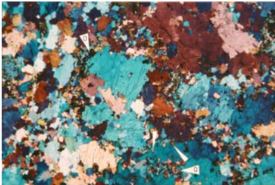
Figure 3. Porphyroclasts of feldspar in a fine-grained, granoblastic matrix of quartz and feldspar. Orthopyroxene inclusions (arrowed) occur in the rims of some plagioclase porphyroclasts and indicate porphyroclast growth into the matrix. Fine-grained opaque minerals (O) are locally abundant and have inhibited growth of the matrix grains. Sample W990772; one wave plate.
