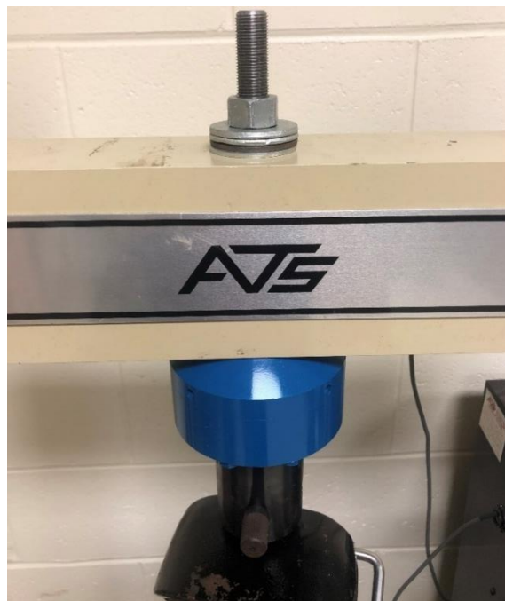
Figure 18: Tensile and flexural tests were performed with an Interface 500 LBS load cell (model 1210AF-500-B)
