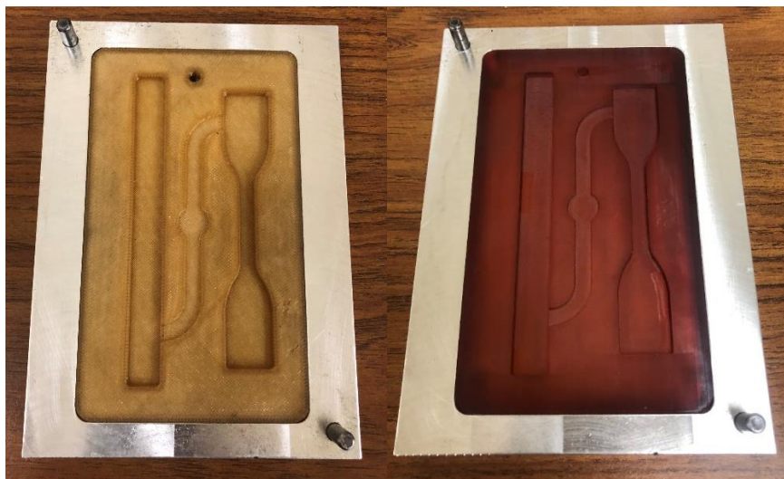
Figure 7: ULTEM 1010 mold insert within the aluminum enclosure (left) and HI-TEMP 300 AMB mold tool within the aluminum enclosure (right)
