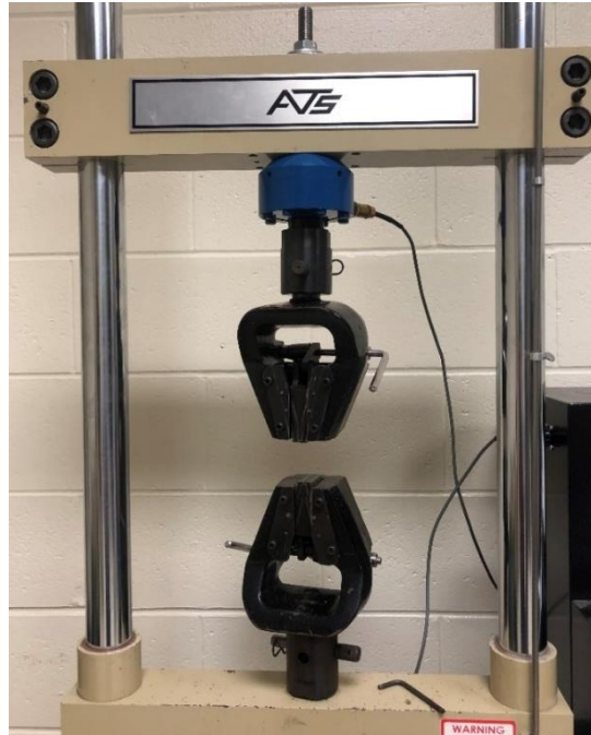
Figure 17: ATS machine with plastic tensile testing grips
