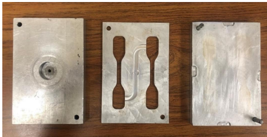
Figure 2: 6061 aluminum 3-piece tensile mold disassembled
