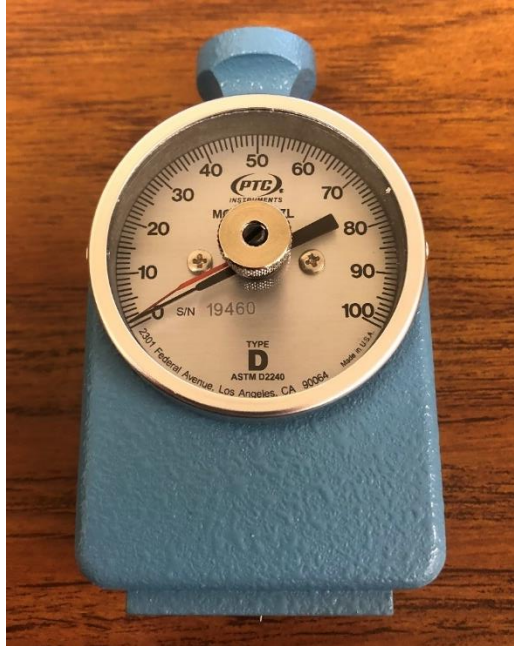
Figure 16: PTC Instruments shore D hardness tester (model 307L)
