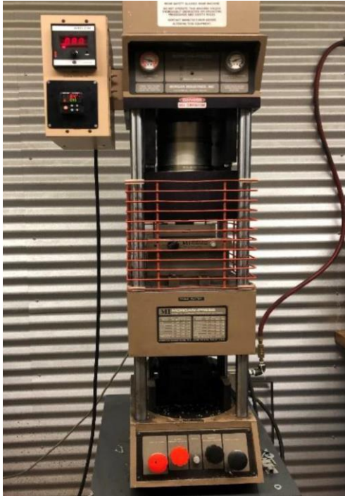
Figure 1: Morgan Press G-125T injection molding machine used for part manufacturing
