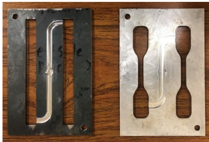
Figure 4: Steel flexural and aluminum tensile center mold tool cutout
