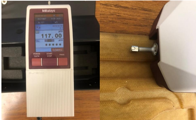
Figure 14: Mitutoyo surface roughness tester (left) and testing the surface roughness of the ULTEM 1010 mold tool (right)
