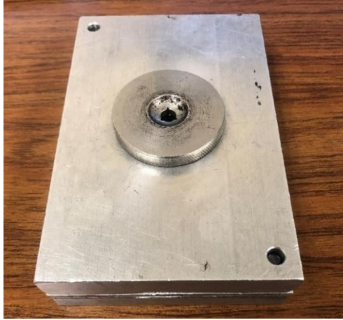
Figure 3: 6061 aluminum 3-piece tensile mold assembled
