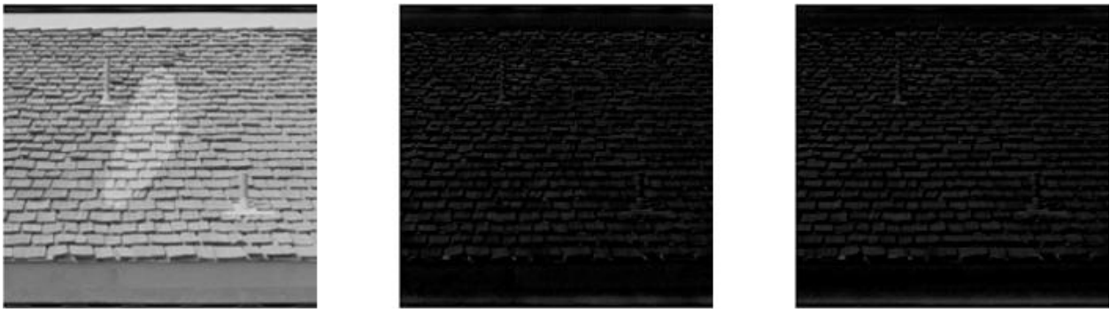
Fig. 3. The image on the left is decomposed with arbitrary \lambda to produce the v image on the center and with optimal \lambda to produce the one on the right. The v image in the center still contains edges at the place of light contrast change (and not just oscillations), and these are gone with the \lambda computed with our approach.
