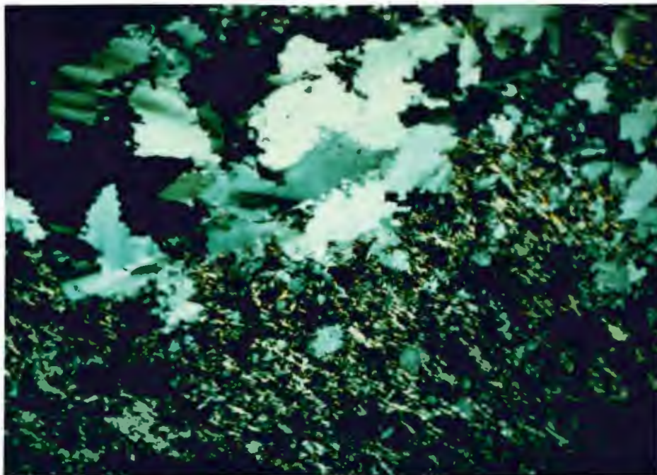
Fig. 85 Large grain of quartz (top) and large sericitized feldspar (bottom) in a deformed granite. Quartz grain has been recrystallized into new grains which show subgrains and detached lobes along serrated grain boundary. Field of view 5 mm. across, polars crossed.
