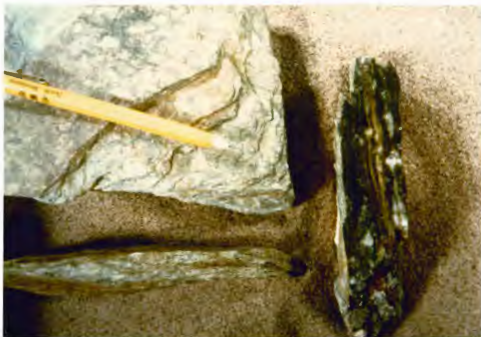
Fig. 10 Layered gneiss phyllonite, samples F-2. Note abundance of dark micas, lineated foliation surfaces (parallel to pencil) and remnant quartz and feldspar porphyroclasts.
