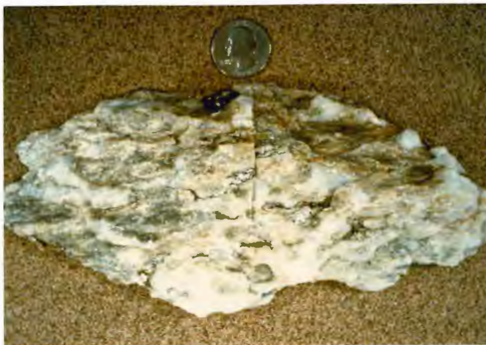
Fig. 33 Deformed and highly sericitized granite. Plagioclase and K-feldspar are completely retrograded to muscovite, and quartz forms white ellipsoidal knots. Sample F-27-5.
