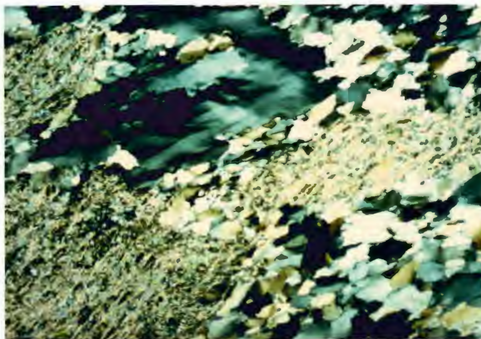
Fig. 36 Photomicrograph of deformed granite from figure 33. Original quartz grains are deformed and recrystallized. Feldspar is completely sericitized and deformed. Field of view is 5 mm. across, polars crossed. Sample F-27-5.
