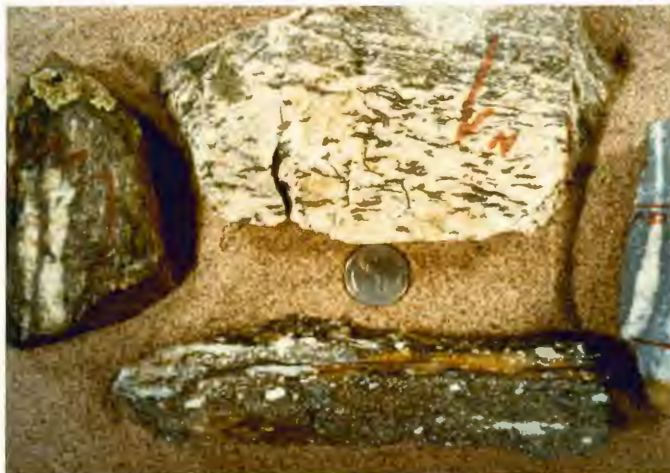
Fig. 19 Samples of retrograde chlorite-epidote gneiss. Clockwise from top samples are F-54-1, F-52-2, F-44-1 and F-52-1. Samples F-54-1 and F-52-1 are little deformed. Samples F-52-2 and F-44-1 are moderately deformed.
