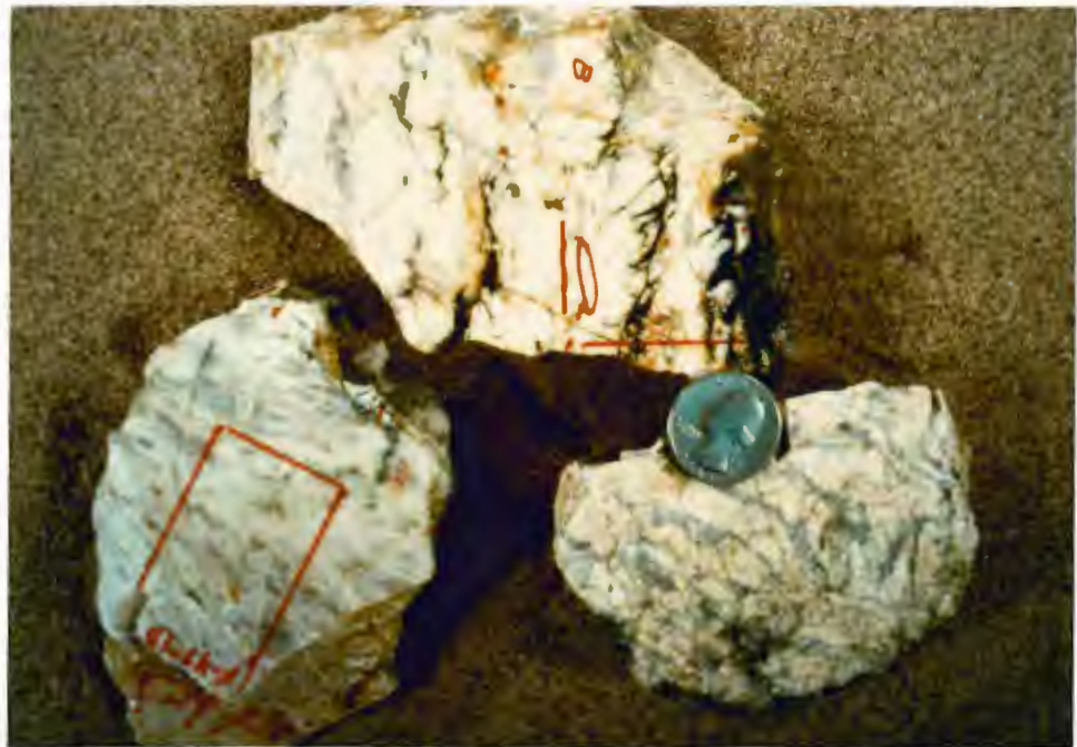
Fig. 32 Samples of deformed granite, F-47-2, F-39-3, F-47-1 clockwise from top. Feldspars acted rigidly while quartz deformed and recrystallized into ribbons. Veins of retrograde minerals have invaded fractures.
