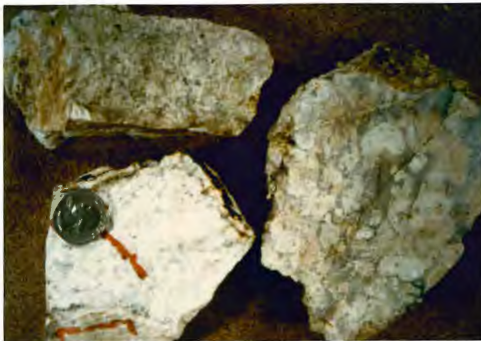
Fig. 27 Samples of least deformed granite, F-51-2, F-51-3, F-27-2, clockwise from right. Variation in color depends on composition, K-feldspar-rich rocks being pinker. Pegmatitic granite on right is mildly deformed.
