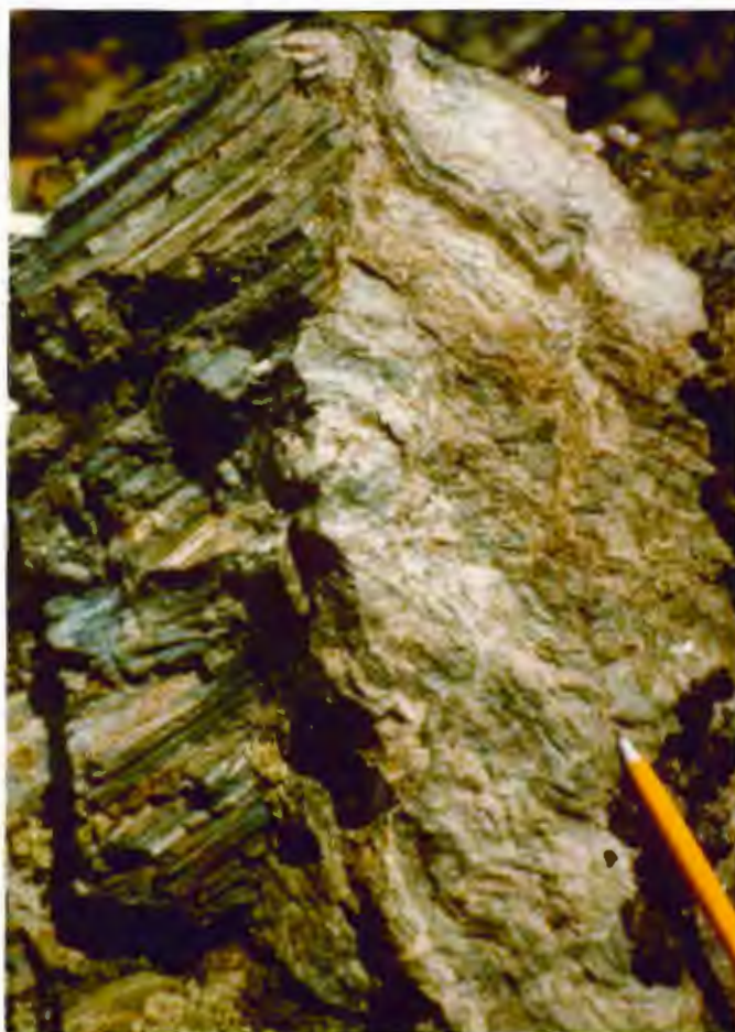
Fig. 68 View looking north at shattered hinge of fold in ultra-mylonite. Rocks are located on east side of FPFZ at PT-31-2. Assymetry of fold suggests transport to east during brittle deformation.
