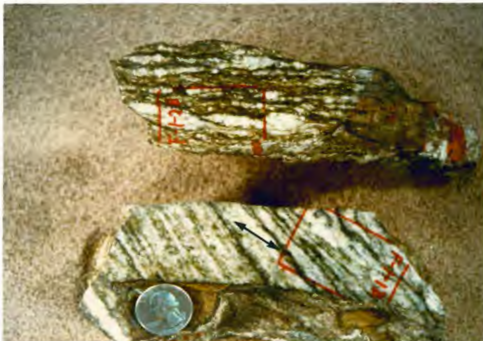
Fig. 9 Mylonitic layered gneisses. Layering in top sample has been disaggregated. Bottom sample is less deformed and has foliation which is oblique to original gneissic layering (note arrow). Samples F-1.
