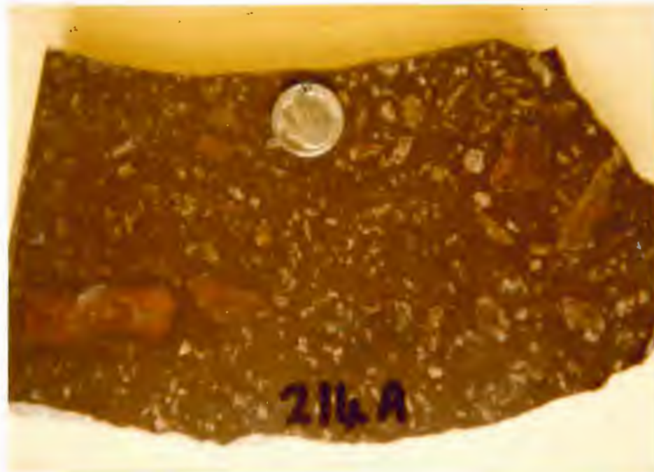
Figure 11: Large, subhedral plagioclase phenocrysts in andesite. Hematite dust gives a reddish color to plagioclase crystals. (Unit LS-2)
