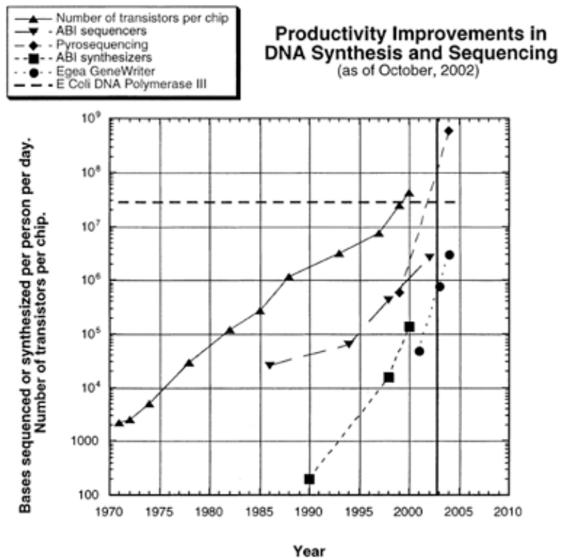
Figure 1.1. Recent Advances in DNA Synthesis and Sequencing Compared with Transistor Integration [Carlson 2003]
