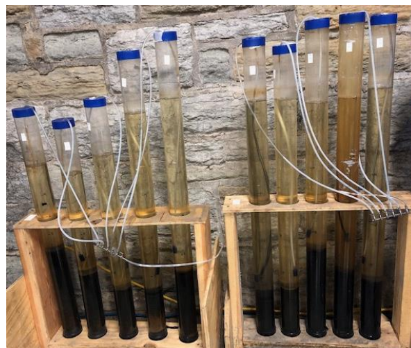
Figure 4. Golden Lake sediment cores set up for phosphorus release study at SAFL.
