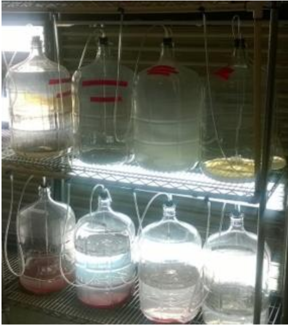
Figure 3. 20 L carboys and fluorescent lamps used in growth of Haematococcus pluvialis .
