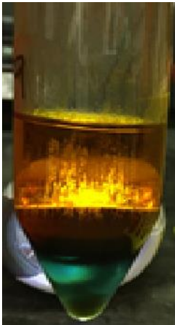
Figure 4. Third extraction of adapted Mojonnier extraction of oil from Haematococcus pluvialis . Upper layer contains algal oil, including astaxanthin.
