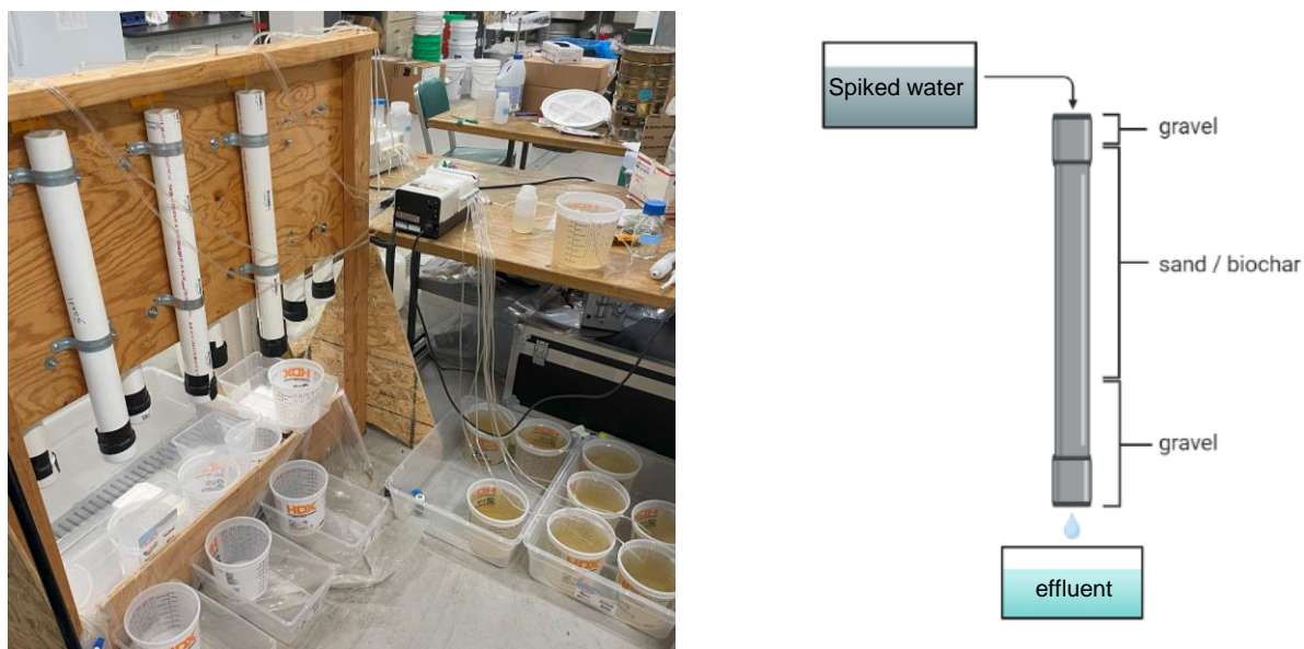
Figure 2.1. A) An image of the column filtration experimental setup. B) A diagram of the makeup of column filters.
