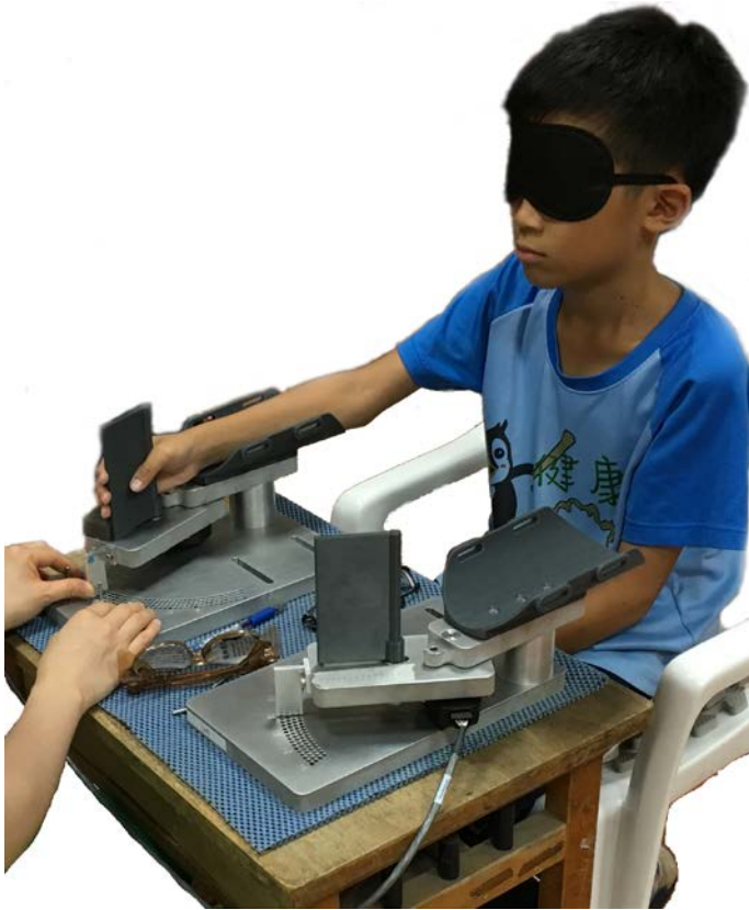
Figure 3. Experimental setup for the psychophysical threshold testing task. Here the experimenter displaced the wrist joint with no active movement of the child.
