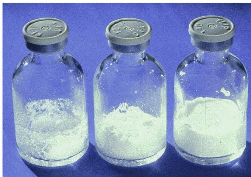
Figure 1.2 Collapsed cake: total collapse (left) and partial collapse (center). The vial on the right shows no evidence of collapse.
