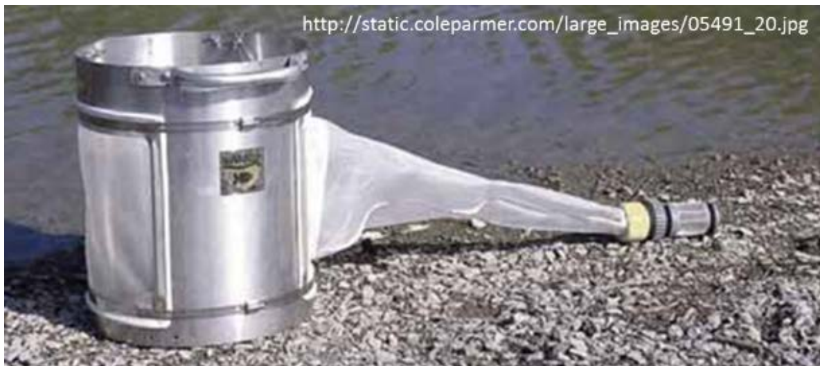
Figure 5. A Hess sampler similar to the equipment used by NRRI. Rocks are thoroughly scrubbed to dislodge macroinvertebrates, which are captured in an attached catch net.
