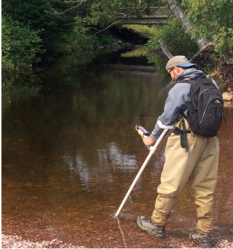
Figure 4. Technician collecting instantaneous temperature data from a MN Lake Superior tributary using a temperature wand constructed at NRRI.
