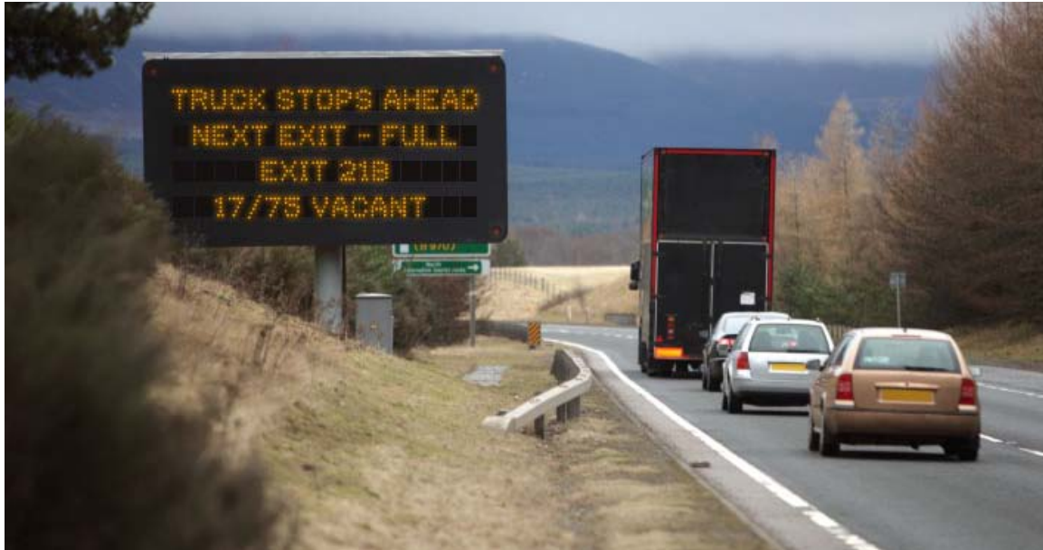
Figure 2 – A sample Variable Message System with live information.
