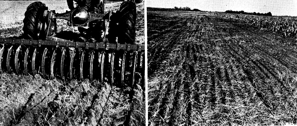
FIG. 9. (LEFT) THE SUBSURFACE PACKER (RIGHT) STRAW MULCH IS SUCCESSFULLY ANCHORED WITH SUBSURFACE PACKER
