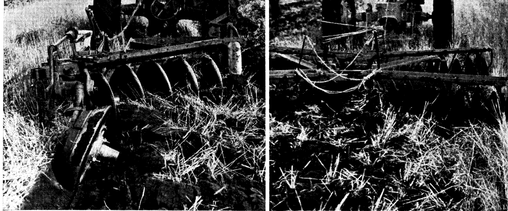
FIG. 6. (LEFT) THE ONE-WAY DISK TILLER LEAVES STUBBLE PARTIALLY ON SURFACE (RIGHT) THE TANDEM DISK LEAVES STUBBLE MULCH ON SURFACE
