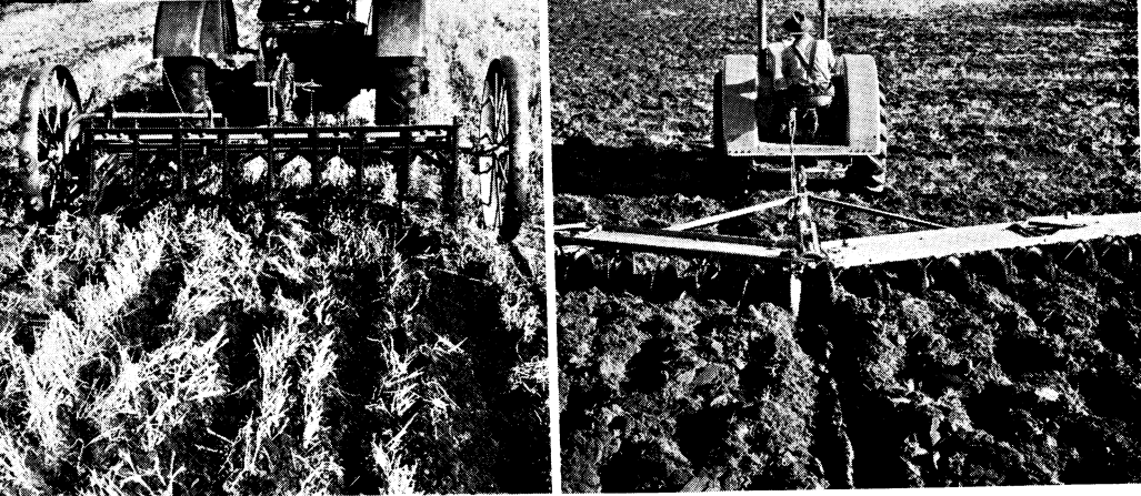
FIG. 7. (LEFT) FIELD CULTIVATOR WITH DUCKFOOT SHOVELS SHOWING WORK IN COMBINE STUBBLE (RIGHT) THE ECCENTRIC OR OFFSET-MOUNTED BASIN DISK
