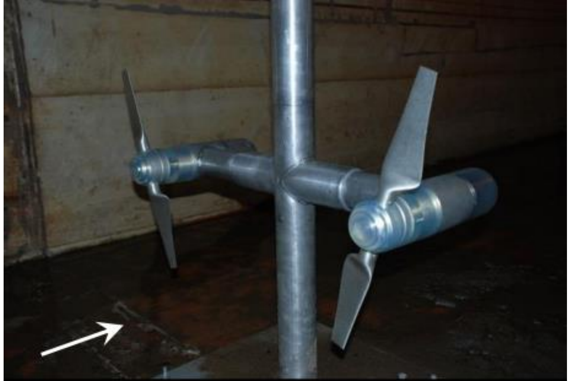
Figure 1. Photo of the scaled RM1 dual-rotor physical model in the UMN SAFL Main Channel. Adapted from [64]. The arrow indicates flow direction.
