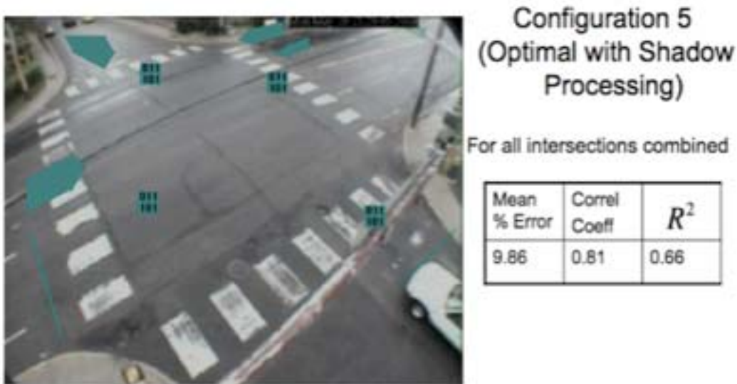
Figure 18: Site 1 – Configuration 5 – combination of presence and directional detectors – one per lane with shadow processing
