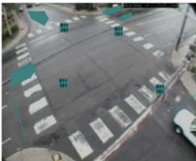
Figure 17: Site 1 - Configuration 4 - combination of presence and directional detectors - one per lane
