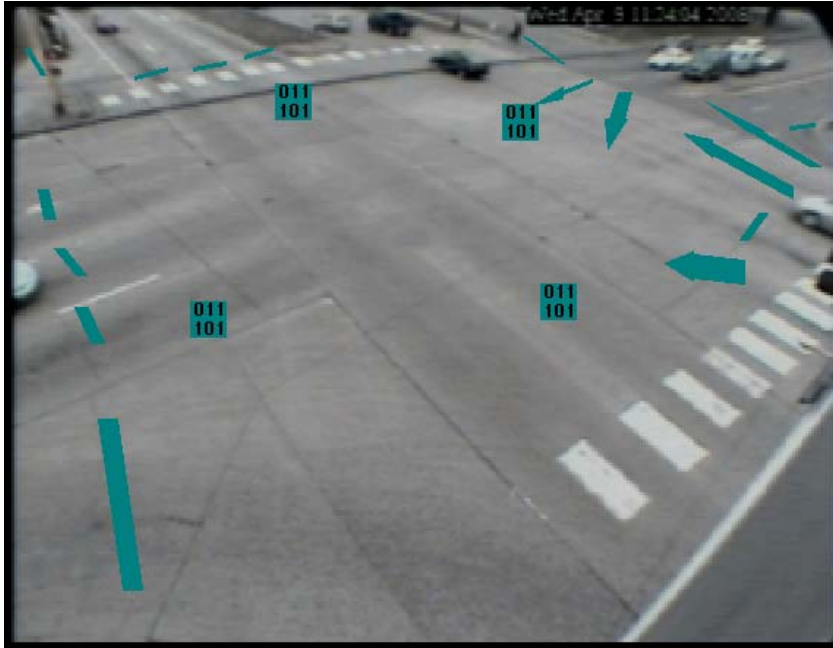
Figure 25: Site 3 - Detector configuration for Snelling Ave. and County Road B (Site 3)
