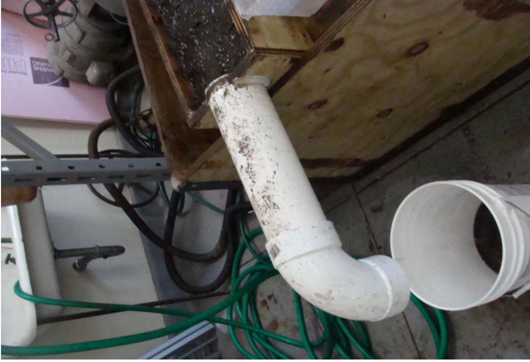
Figure 3.5. Total runoff collection in 5 gal bucket
