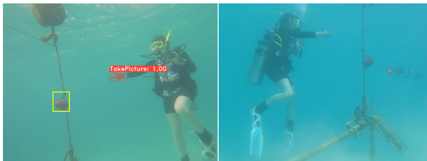
Figure 5.1: Demonstration of the SPOC communication method in the Caribbean Sea. The LoCO AUV has located the object of interest (yellow box) and received instruction from the diver in the first image. The red light on the AUV in the second image means it received the task “Take a Picture”.
