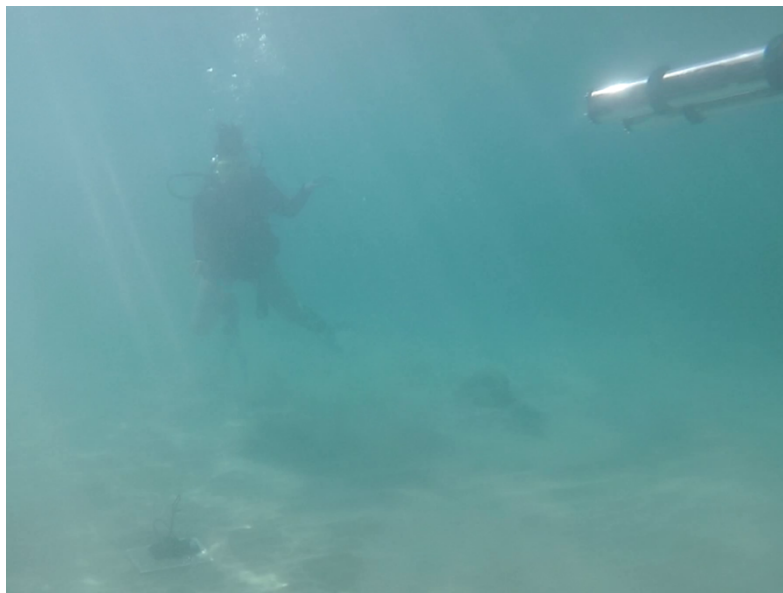
Figure 3.1: The LoCO AUV running DIP to navigate towards an object we point at on the seabed in response to diver pointing gesture. Image taken during field test in the Caribbean Sea.
