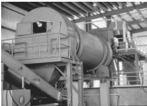
Shown above is the Hutchinson project's mixing vessel, where source separated organics are mixed with woodchips.
