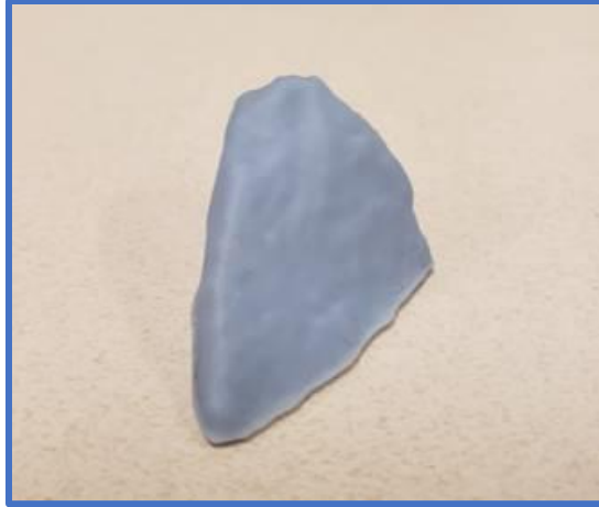
FIGURE 18. First Prototype 3D-Printed ISO Fine Particle Model
