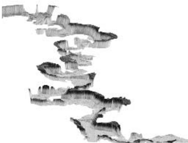
Laser scan of two riverbanks on the Blue Earth River.
