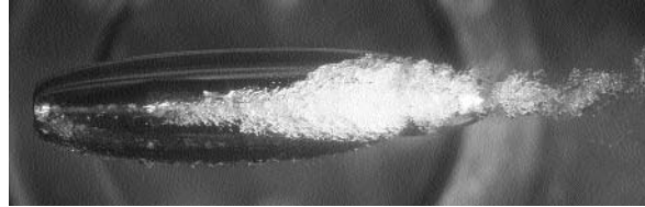
Ventilated test body.
