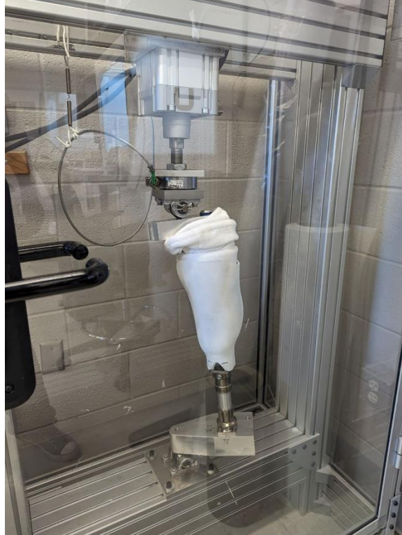
Figure 6. Experimental setup for ISO 10328 P6 Condition II ultimate strength test (Socket A).
