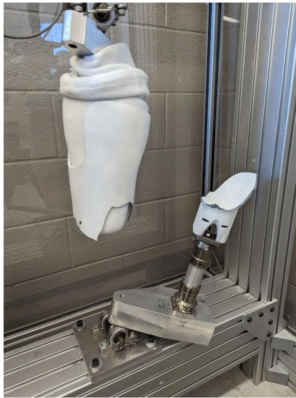
Figure 10. Failure mode for Socket C.
