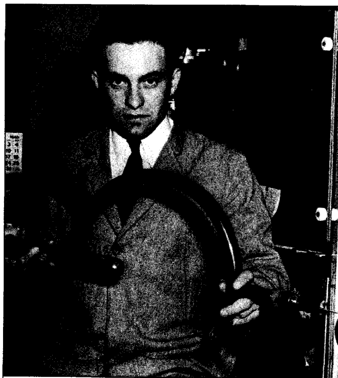
Alfred O.C. Nier, 29, with the mass spectrograph tube he used to isolate the first sample of uranium-235 in 1940. The tube is now in the Smithsonian Institution in Washington, D.C.
