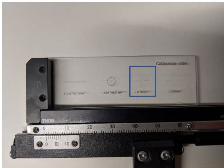
Figure B.1: Slide used for calibrating the experimental technique used in this study
