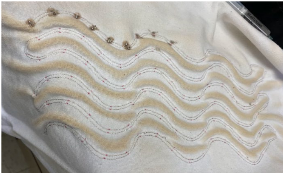
Figure 29 - Scorched fabric substrate
