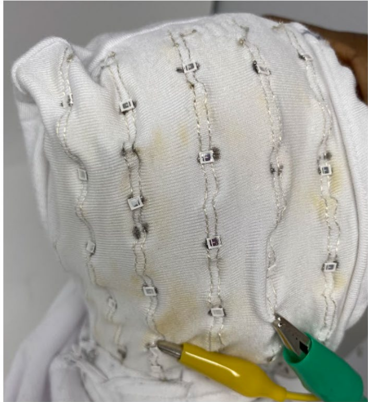
Figure 26 - (left) Serpentine rows layout of 2 parallel stitched traces (power and ground) (right) soldered, stitched traces on the hoodie pattern piece
