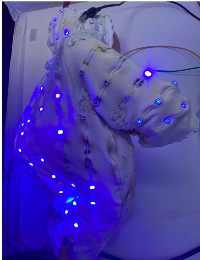
Figure 27 - LEDs powered by a single power source before the supply voltage was high enough to illuminate all of them
