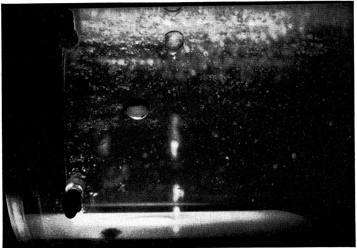
Fig. 5 - Cavitation in Diverging Closed - Jet Test Section with Diffuser Transition
