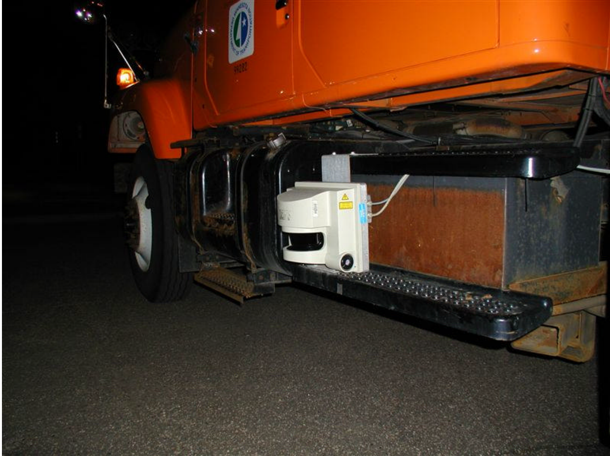
Picture 2-1. Picture of Sick LMS 221 mounted on left side of Safeplov research vehicle. The Safeplov was used as the trailing vehicle during on-road testing.
