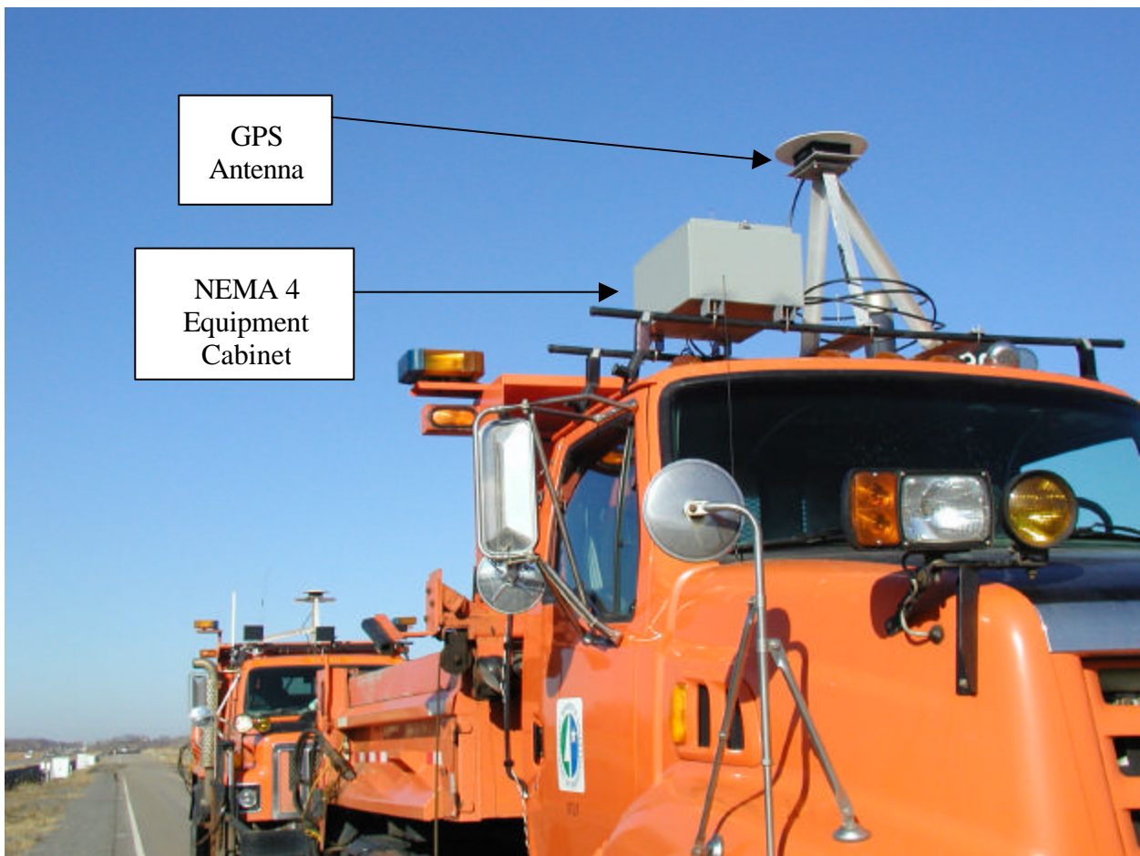
Picture 3-1. Photo of lead snowplow showing location of DGPS antenna and NEMA 4 cabinet in which all necessary equipment resides.
