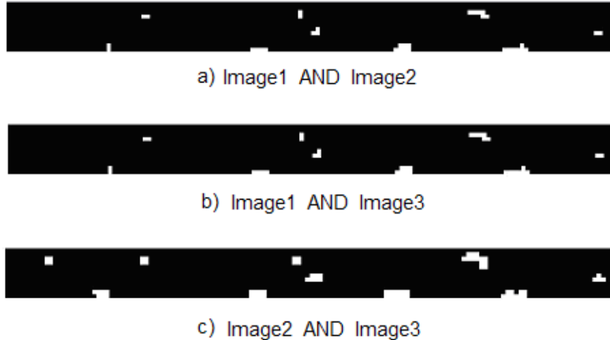
Figure 4.5 Common Objects Taken From Pair of Binary Images a) New_Image1 = Image1 AND Image2 b) New_Image2 = Image1 AND Image3 c) New_image3 = Image2 AND Image3
