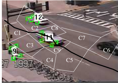
Figure 2.1: Example cell-based representation of the spatial region. The cells are shown as white regions with the corresponding labels. An example trajectory of a lane-changing vehicle is shown in black.
