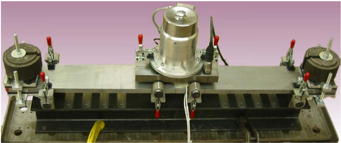
Fig. 5.8. Testing setup for the BVT with additional damping
