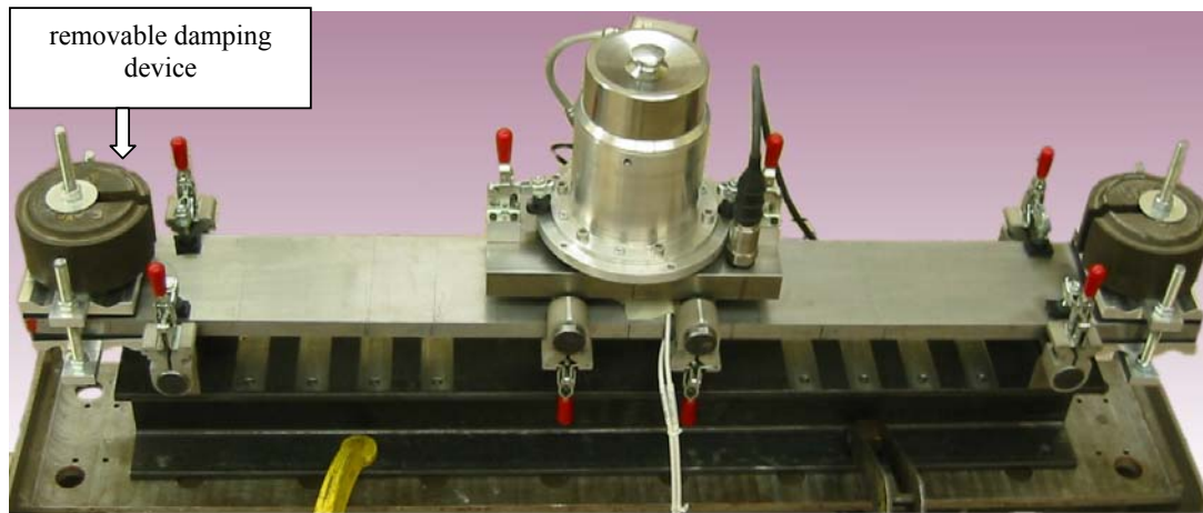
Fig. A.1.3. Testing setup for the BVT with damping devices
