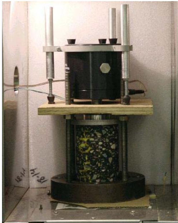
Figure 5.2. Vibration Test Setup
