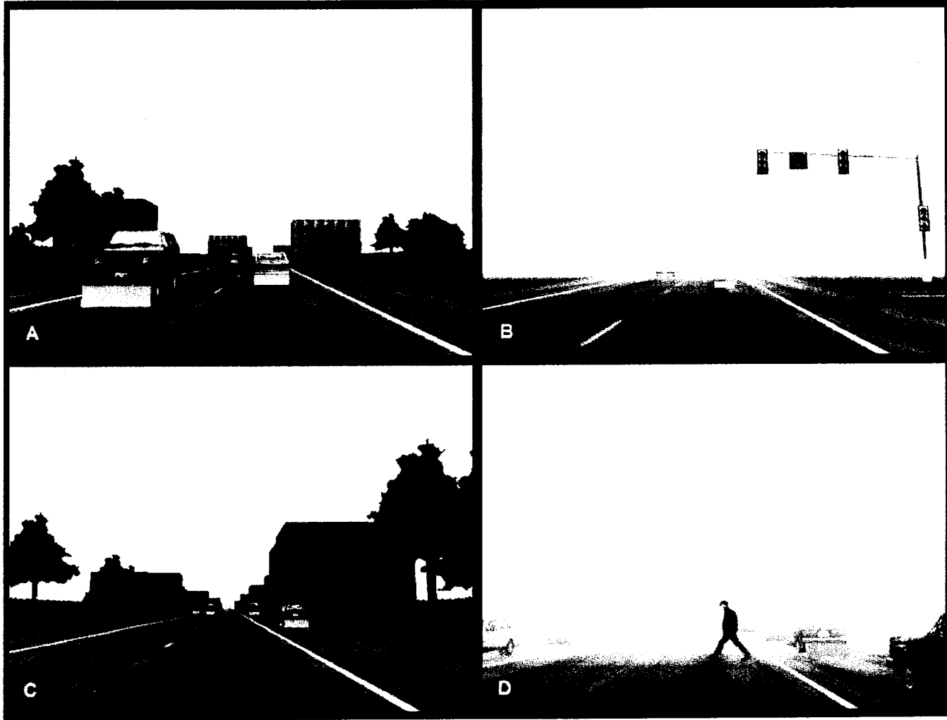
Figure 4.2. Traffic scenarios used in the study: A, follow the lead car and brake in a 2 s gap; B, respond to lights and intersection traffic appropriately; C, everyday driving through city streets; and D, the sudden appearance of a pedestrian which requires braking and steering to avoid.
