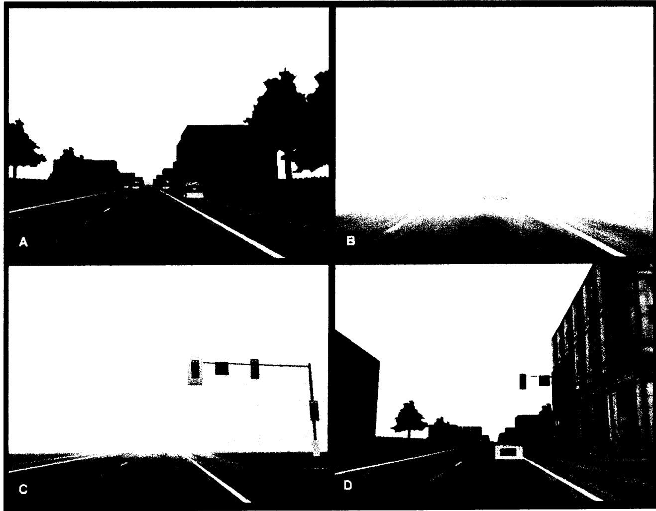
Figure 4.1. Examples of conformal (A and C) and non-conformal VES displays (B and D). Conformal displays are overlaid directly onto traffic environment elements such as other vehicles (A) and stop lights (C). Non-conformal displays are coupled to the traffic elements such as other vehicles (B) and stop lights (D), but the information always appears centered on the roadway (B & D).
