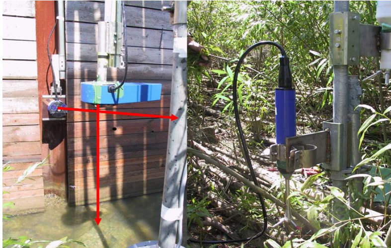
Figure 8.8 Measuring devices: acoustic Doppler profiler (left), acoustic Doppler velocimeter (right).
