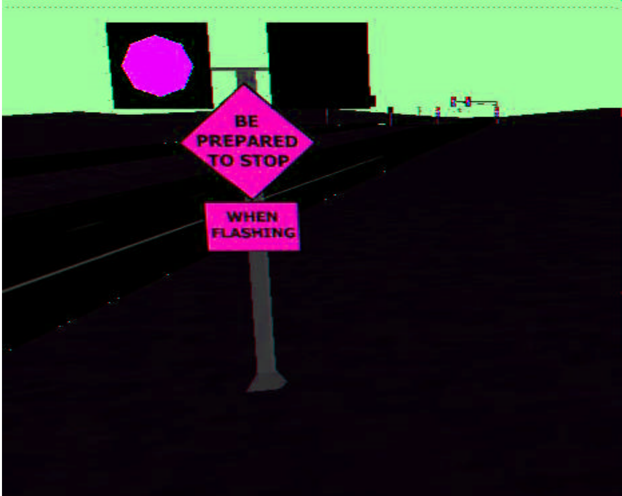
Figure 2-3. Perspective from SDTE showing simulated AWF in foreground, and simulated pole and mast arm with dual traffic signal in background.
