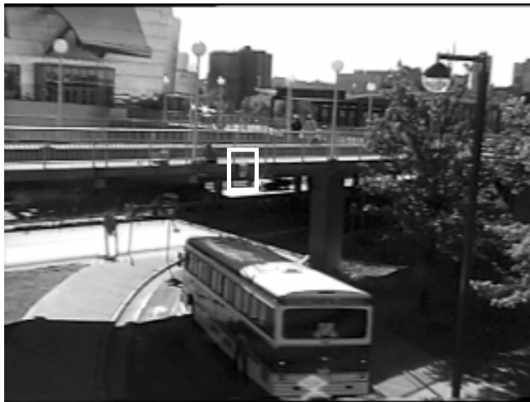
Figure 23: A view of the AUTOSENSE II sensor as a bus passes underneath it (the sensor is shown highlighted with a white box around it).
