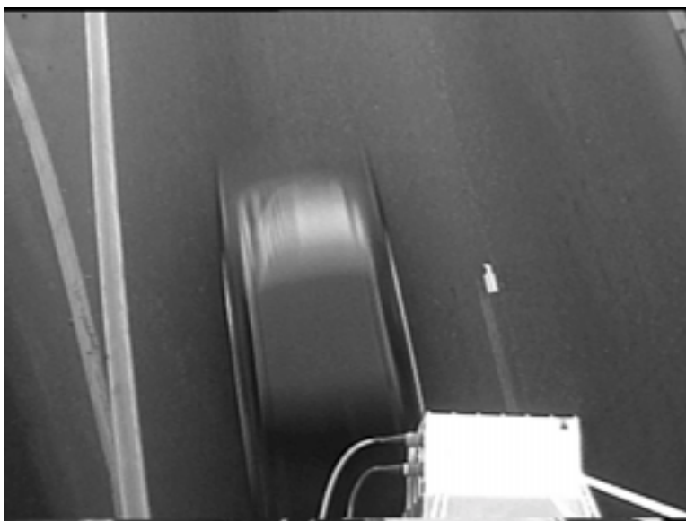
Figure 26 : Image of traffic as seen by the AUTOSENSE II sensor as a car passes underneath it.
