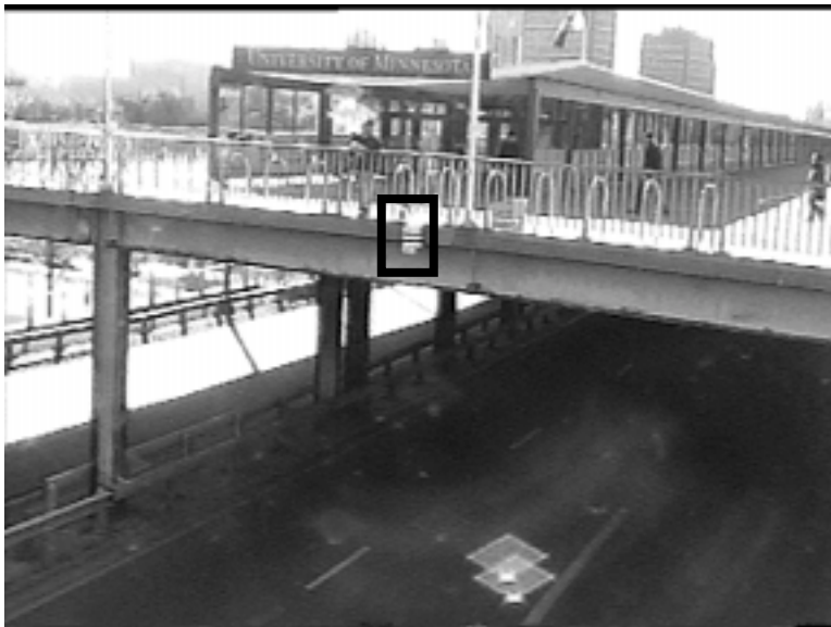
Figure 25 : The AUTONSENSE II sensor mounted above Washington Ave. (sensor is highlighted with a black box around it).
