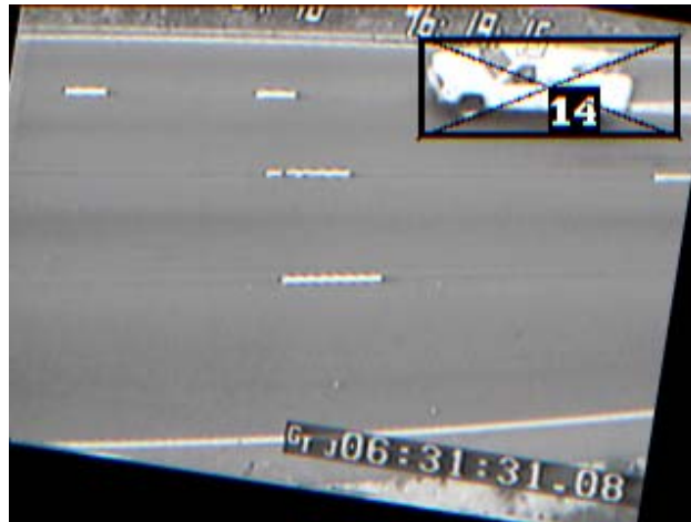
Figure 9 : Identification and classification of the vehicle.
