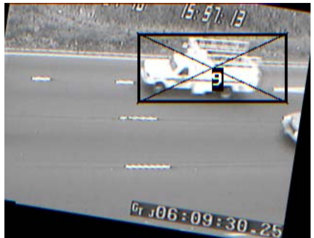
Figure 11 : Correct classification of a truck.
